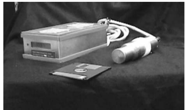
FIGURE 8-4 The Tissue Equivalent Proportional Counter (TEPC) is an automatic microdosimetry system, which consists of a spectrometer unit and a detector unit. The spectrometer unit contains a computer that allows real-time analysis of the data and provides data on the dose equivalent rate as a function of lineal energy ( y ) and time for space radiation. The TEPC is filled with a low-pressure gas. TEPCs are also used in aviation.
